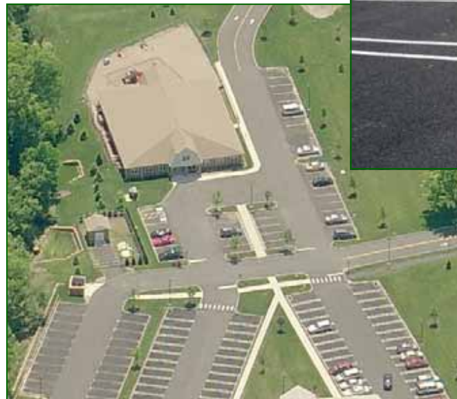
Above: Porous pavement shown at left and conventional pavement to the right in the parking facility at the Doylestown Commerce Center.
