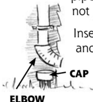
Insert downspout INTO the elbow and attach using sheet metal screws and predrilled holes. (Do not insert the elbow up inside the downspout or it will leak).
