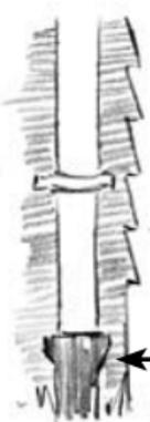
Using a hacksaw, cut your downspout approximately 9 inches above the sewer standpipe, or if installing a rainbarrel, make your cut above the barrel according to the manufacturer's instructions.
